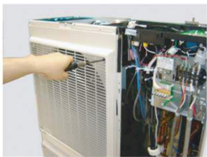
Remove the 4 mounting screws.
