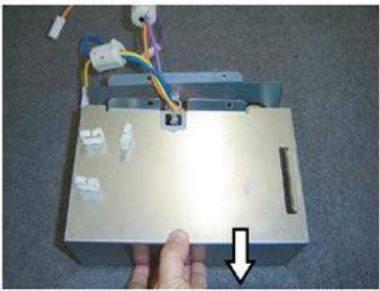
Remove the CONDENSER COVER by sliding toward.
