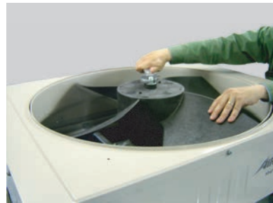
Remove the nut. Note the tightening torque at the installation. Tightening torque is from 15 to 20N·m.
