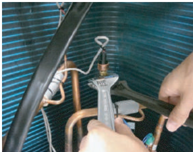
Remove the PRESSURE SENSOR with wrench.
