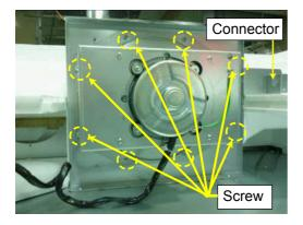
4: Turn 8 pieces of screw on the Motor ASSY and remove the wired connector.
