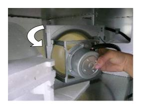
6: Rotate the Motor ASSY around the axis. (Note) Actually, The color of a wheel is black.
