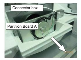
3: Pull the partition board A out to the direction of arrow.
