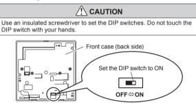
Before using this product, always set DIP switch to "ON". If not set, when the main power is turned on again, the set data by menu operation will be erased and cause erroneous operation.
