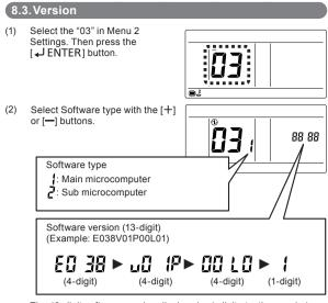
The 13-digit software version displays by 4-digit at a time each 4 seconds
