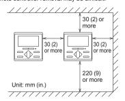
\* Please secure enough space where a flat-blade screwdriver to take off a case can be inserted.
