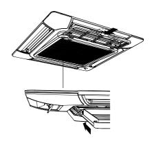
5. Close the intake grille and push the intake grille's hooks outward.
