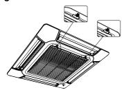
2. Pull out the filter from the intake grille.
