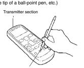
To end test operation, press the remote control unit START/STOP button. (When the air conditioner is run by pressing the test run button, the OPERATION indicator lamp and TIMER indicator lamp will simulta-
