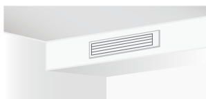
Closed louver [Operation is stopped.]
