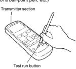
To end test operation, press the remote control unit START/STOP button (When the air conditioner is run by pressing the test run button, the OPERATION indicator lamp and TIMER indicator lamp will simulta-
