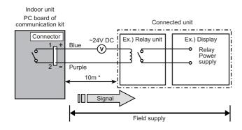
\* Make the distance from the PC board to the connected unit within 10m. Relay spec. : Max.24V DC, 10mA to less than 500mA.
