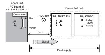
\* Make the distance from the PC board to the connected unit within 10m. Relay spec. : Max.24V DC, 10mA to less than 500mA
