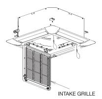
⑥ Close the INTAKE GRILLE, and hook the loop of the HOOK WIRE to the attached screw at step ③ (left and right 2 positions).
