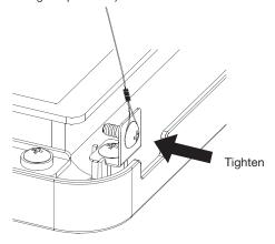
(8) Close the INTAKE GRILLE so that the HOOK WIRE is not fasten, and then, close the GRILLE HOOK.
