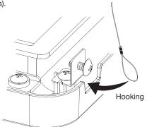
Tasten the HOOK WIRE and tighten the screw till the end. (left and right 2 positions).
