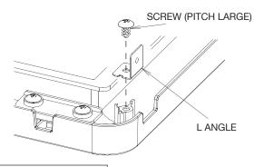
Tightening torque 0.8-1.2N·m (7.1-10.6in. lbs)
