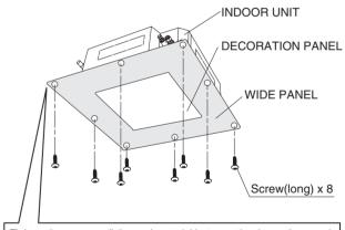
Tighten the screw until the seal material between the decoration panel and the main indoor unit is compressed to a thickness of 5-7mm
