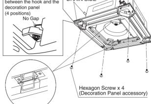
When there is a gap between the ceiling and the decoration panel even when the screw is tightened, readjust the height of the main indoor unit
