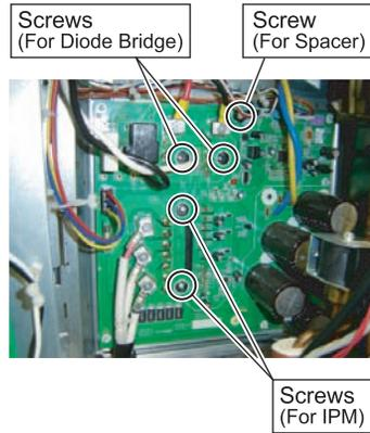
Remove the 5 mounting screws.
