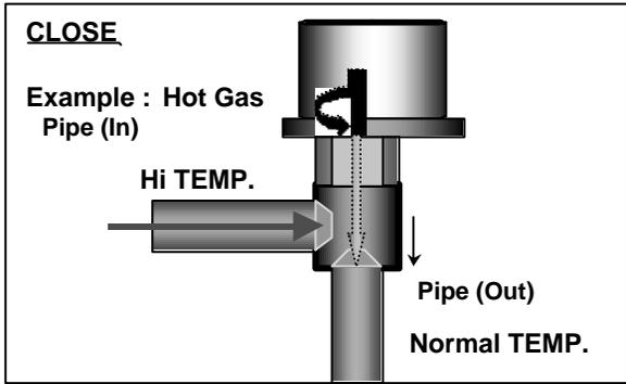
If it is open, it has no temp. difference between Inlet and Outlet.
