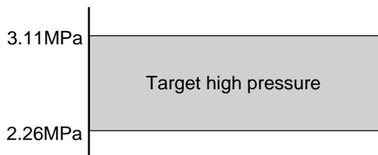
( Fig. 4 : Target high pressure range for MIN. HEAT OPERATION)
