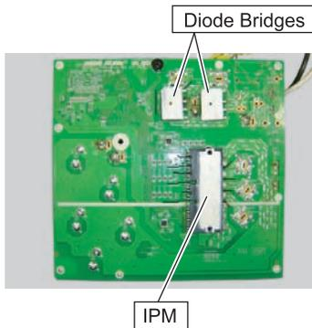
Spread the Heat Transfer Compound on the other side of IPM and Diode Bridges when you exchange INVERTER PCB by the repair.
