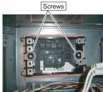
Remove the 2 mounting screws.
