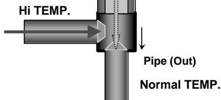
If it is open, it has no temp. difference between Inlet and Outlet.
