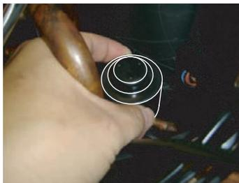
Remove the EEV COIL by hand.
