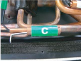
Remove the THERMISTOR SPRING with the THERMISTOR.
