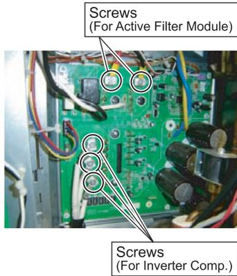
Remove the 5 mounting screws and wires.
