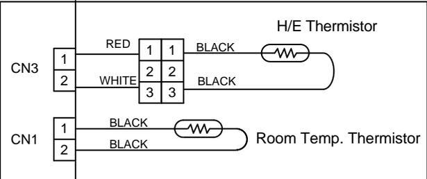
► **If the voltage does not appear, replace Controller PCB and execute the check operation again.**
