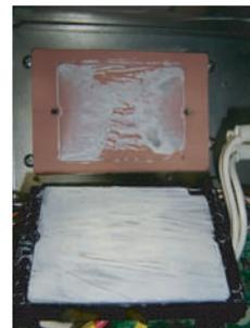
Spread the Heat Transfer Compound on the other side of Active Filter Module when you exchange Active Filter Module by the repair.
