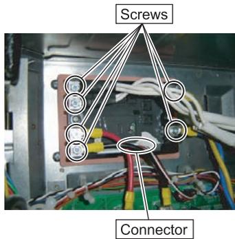
Remove the 6 mounting screws and wires.
