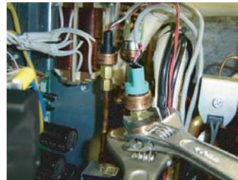
Remove the PRESSURE SENSOR with wrench.
