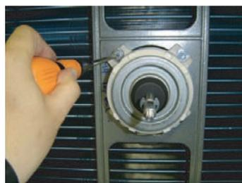
Remove the 4 mounting screws.
