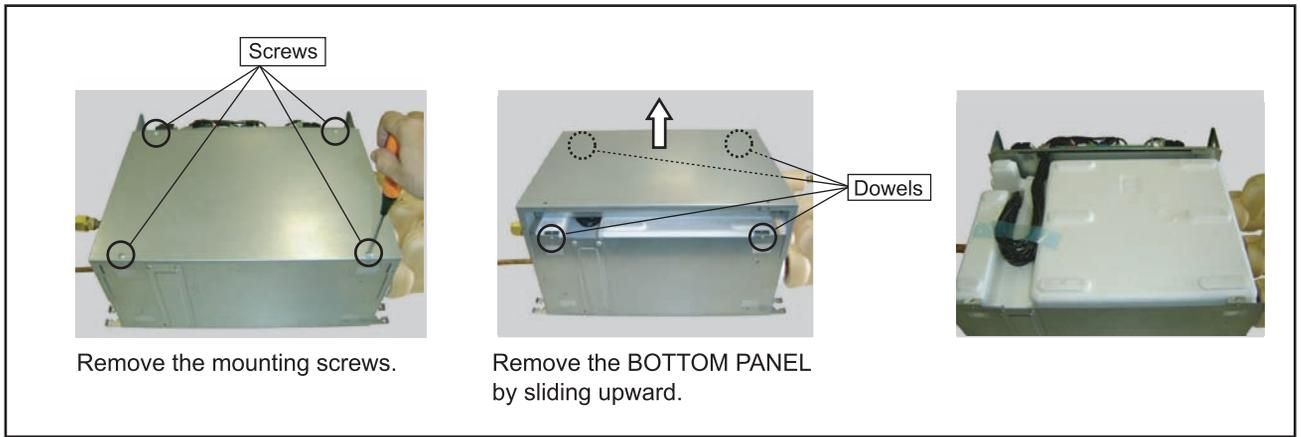
Remove the mounting screws.
