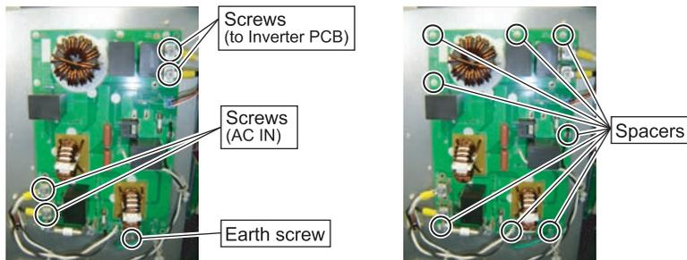
Remove the connector and screws.
