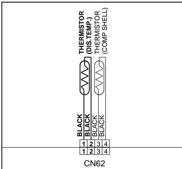
Discharge temperature thermistor (CN62:1-2)
