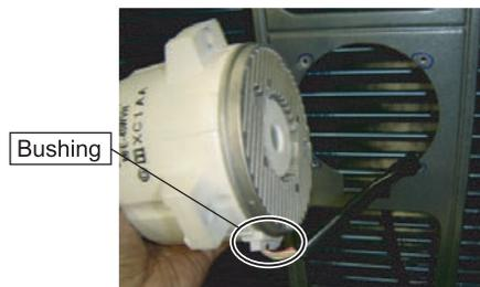
Remove the FAN MOTOR.
